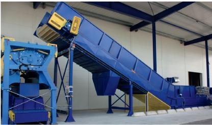
Our range of feeding conveyors and hoppers makes it possible to regulate perfectly the input flow in our installations. We offer different hopper technologies that, depending on weight, volume, density and stored material, fit your needs. This help to increase efficiency and purity during the sorting steps.
