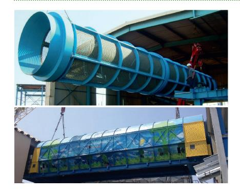
The choice of a trommel is defined by our engineers, depending on the nature of the products to be treated, the flow and the sorting process. Our range of rotary trommel or drum screen is available in different diameters and lengths according to your needs. Alfyma realize and install trommel among the biggest in Europe which can process MSW or up to 40,000 tons of PET plastic bottles per year.
